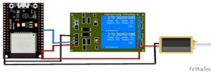
Gambar 5. Rangkaian Koneksi ESP32-Relay-Solenoid Lock Door
