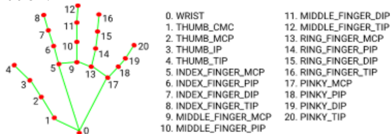
Figure 5. MediaPipe Hand Landmarks Coordinates Explanation [19]
