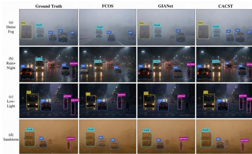
Figure 2. Qualitative detection comparisons on diverse adverse conditions: (a) Dense Fog, (b) Heavy Rain at Night, (c) Extreme Low-Light, (d) Sandstorm. CACST consistently localizes objects missed or falsely detected by specialized baselines.
