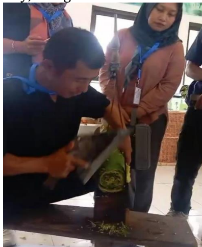
Figure 1. Conventional tobacco shredding process
