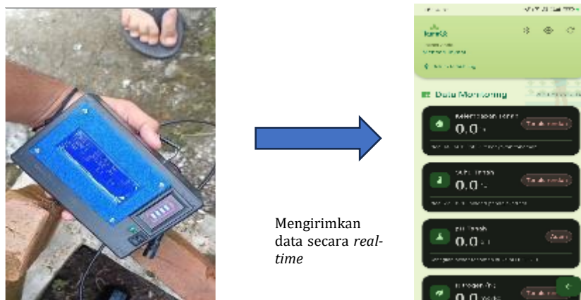
Gambar 6. Hardware dan Software Monitoring Nutrisi Kandungan Tanah
